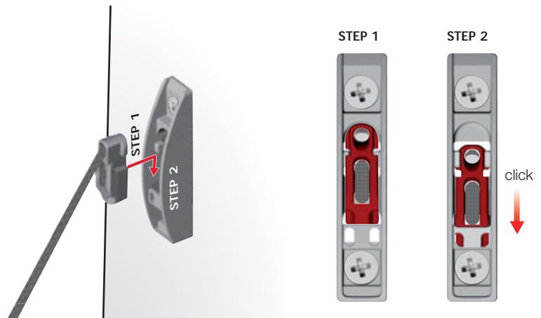
Lift the door almost completely to slot the end element of the wire into the door bracket.
