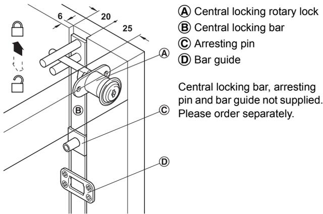
Mount central locking rotary lock on the right hand side.
