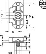
For continuous profile rod Ø 6 mm or 8 mm, for cylinder cores that are
